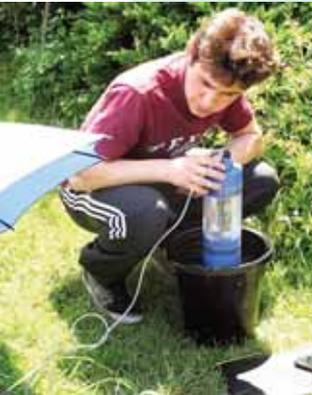
Martin is sampling the groundwater aquifer in the Kempton Park Gravels that lie under the allotments and which feed our water pumps. The closely spaced series of pumps/boreholes allows an assessment of variation across the site, which could be related to the
